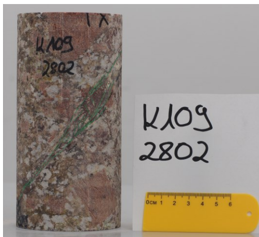
Figure 1: One example of fracture observed in drill-core from Soultz-sous-Forêts. Interpreted microcracks are drawn in green lines.
